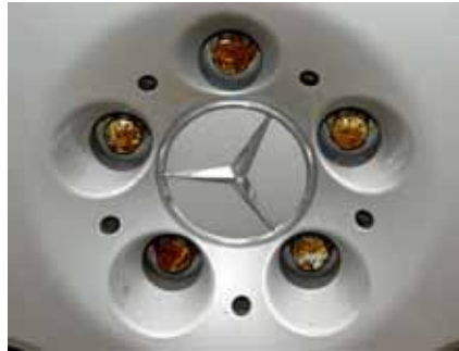
The wheel nuts or wheel bolts show clear signs of rust, but they are not round and can be detached.
