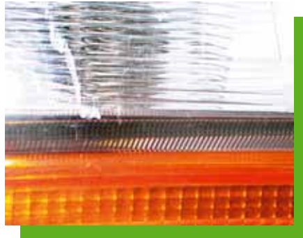
Tears or smaller breaks in lightings not influencing the function or vehicle safety.
