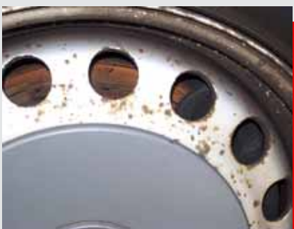
Deformation of the bead of the rim, missing material or rust.
