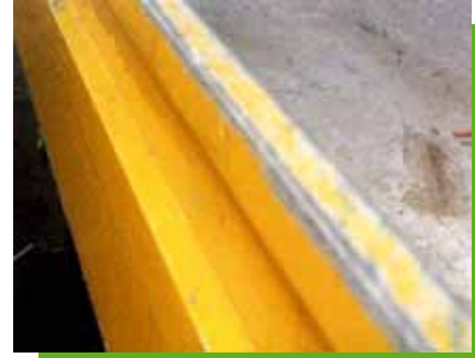
Abrasions on the sills of back or sides doors of the loading compartment caused by loading of goods.
