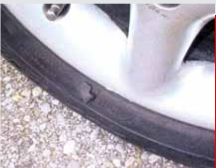
Tyre with damage caused by impact known to happen through 'kerbing'.
