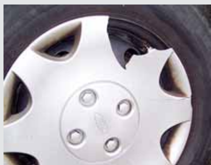
Breaks or missing material on wheel caps. Scuffing and scratches causing a deformation of the wheel cap.
