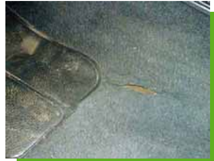
... There are abrasions, discolourings and tears in the most used areas.
