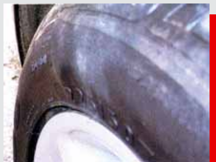
Clearly visible dents caused by breaks in the sidewalls of the tyre or missing material.
