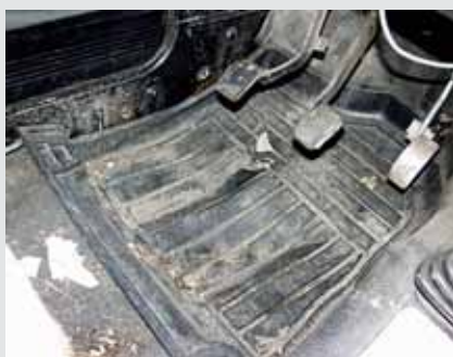
The vehicle carpet shows clear tears, holes or visible stains and dirt marks.
