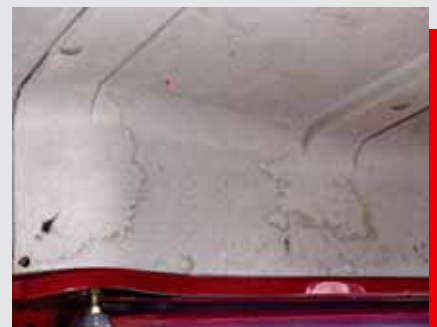
Panel headlinings are deformed or show cuts in material or are heavily stained.
