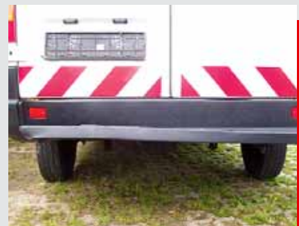
Damages from impacts in the area of the loading compartment. Deformed sills or broken material of the sills.
