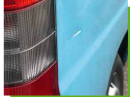
Scuffing or scratches even with damages to the paint, if the diameter does not exceed 20 mm each (size of the 1 Euro coin).
