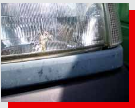
Chippings in the headlights, fog lights or indicators having broken the glass or the transparent covers.
