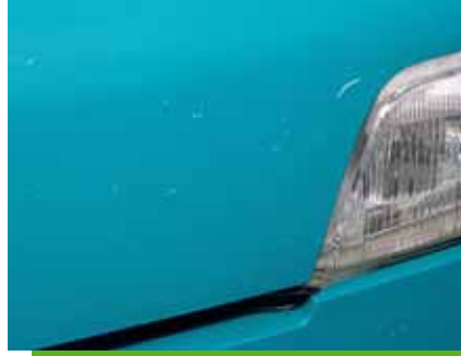
Scuffing or scratches with a maximum length of 100 mm.
