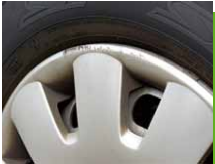
Scuffing or scratches or deposits on rims not deforming the rim.
