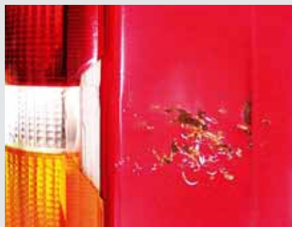
Scuffing and scratches through to the metal or substantially influencing the optical condition of the vehicle by their number on one body part.
