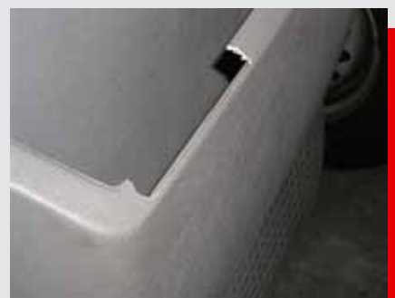
Storage areas in the doors or at the dashboard are torn or material is broken.
