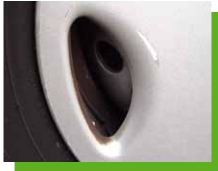
Scuffing or scratches on wheel caps not causing breaks in the material or deforming the wheel cap.
