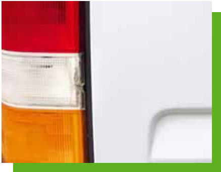
Tears or smaller breaks in indicators or number plate lights not influencing the function or vehicle safety.
