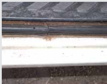
Damages to body parts or paint in the area of the loading compartment causing rust.
