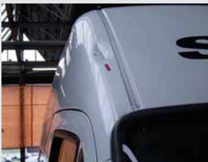
Deformation of the vehicle body with or without damages to the paint with a diameter of more than 20 mm each (size of the 1 Euro coin).
