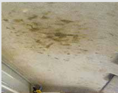
The headlining of the driver cabin is stained. The staining is not only on the surface and cannot be removed by normal cleaning. The material or its seams are torn.
