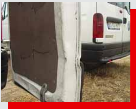
Deformation of body parts, partition walls, doors or windows.
