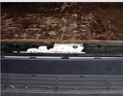
Rips or tears or missing parts on the loading floor or lining in the area of the loading compartment.
