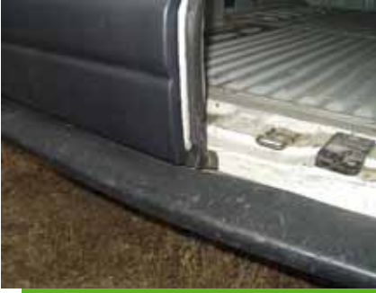
Scuffing and scratches or abrasions on sills of loading compartments or bumpers in that area.
